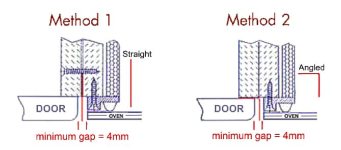
**Note**, failure to install heat deflectors in either method voids the warranty.
